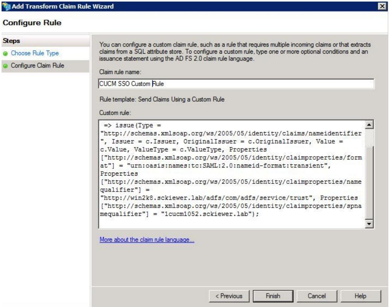
The screenshot shows the 'Add Transform Claim Rule Wizard' dialog box, specifically the 'Configure Rule' step. The 'Steps' pane on the left shows 'Choose Rule Type' and 'Configure Claim Rule' (which is selected). The main area contains the following text:
