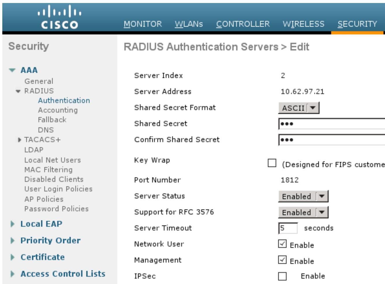
The screenshot shows the Cisco WLC configuration interface. The top navigation bar includes 'MONITOR', 'WLANs', 'CONTROLLER', 'WIRELESS', and 'SECURITY'. The left sidebar shows the 'Security' menu with 'AAA' expanded to 'RADIUS' > 'Authentication'. The main content area is titled 'RADIUS Authentication Servers > Edit' and displays the following configuration details:
