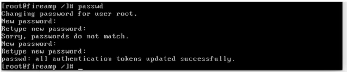
A terminal window showing the execution of the 'passwd' command. The output indicates that the password for the 'root' user is being changed, followed by prompts for a new password and its retype. An error message states 'Sorry, passwords do not match.' followed by a successful completion message: 'passwd: all authentication tokens updated successfully.'
