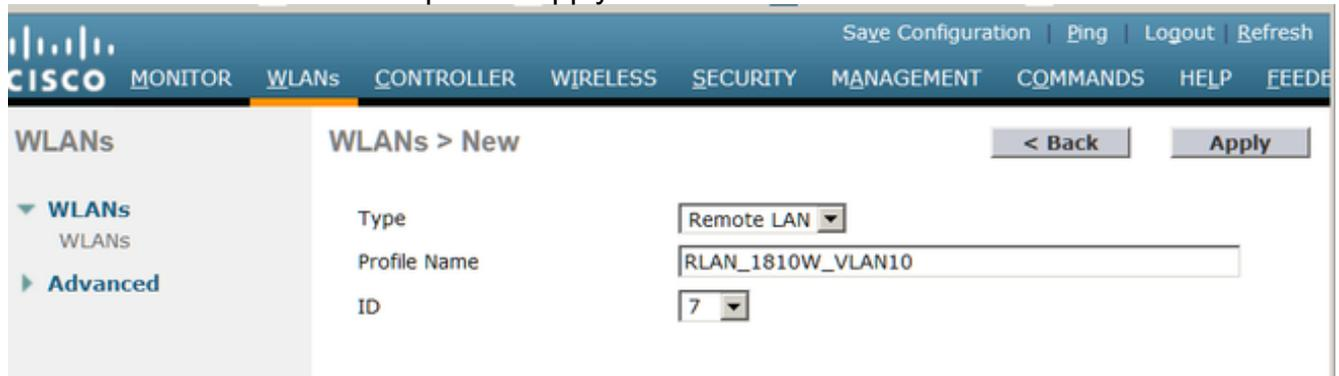
The screenshot shows the Cisco WLC configuration interface for creating a new RLAN. The page title is "WLANs > New". The "Type" is set to "Remote LAN", the "Profile Name" is "RLAN\_1810W\_VLAN10", and the "ID" is "7". There are "Back" and "Apply" buttons.
