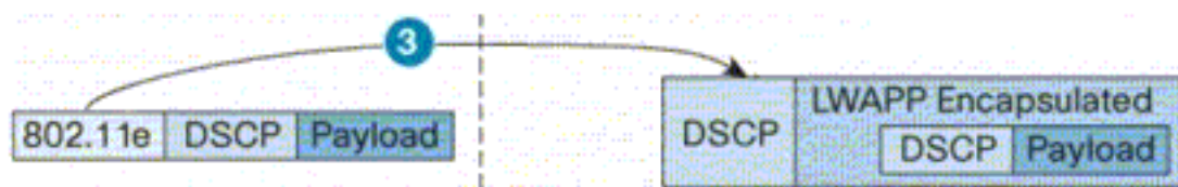
802.11e UP value translated to DSCP value af41 and sent to Controller
