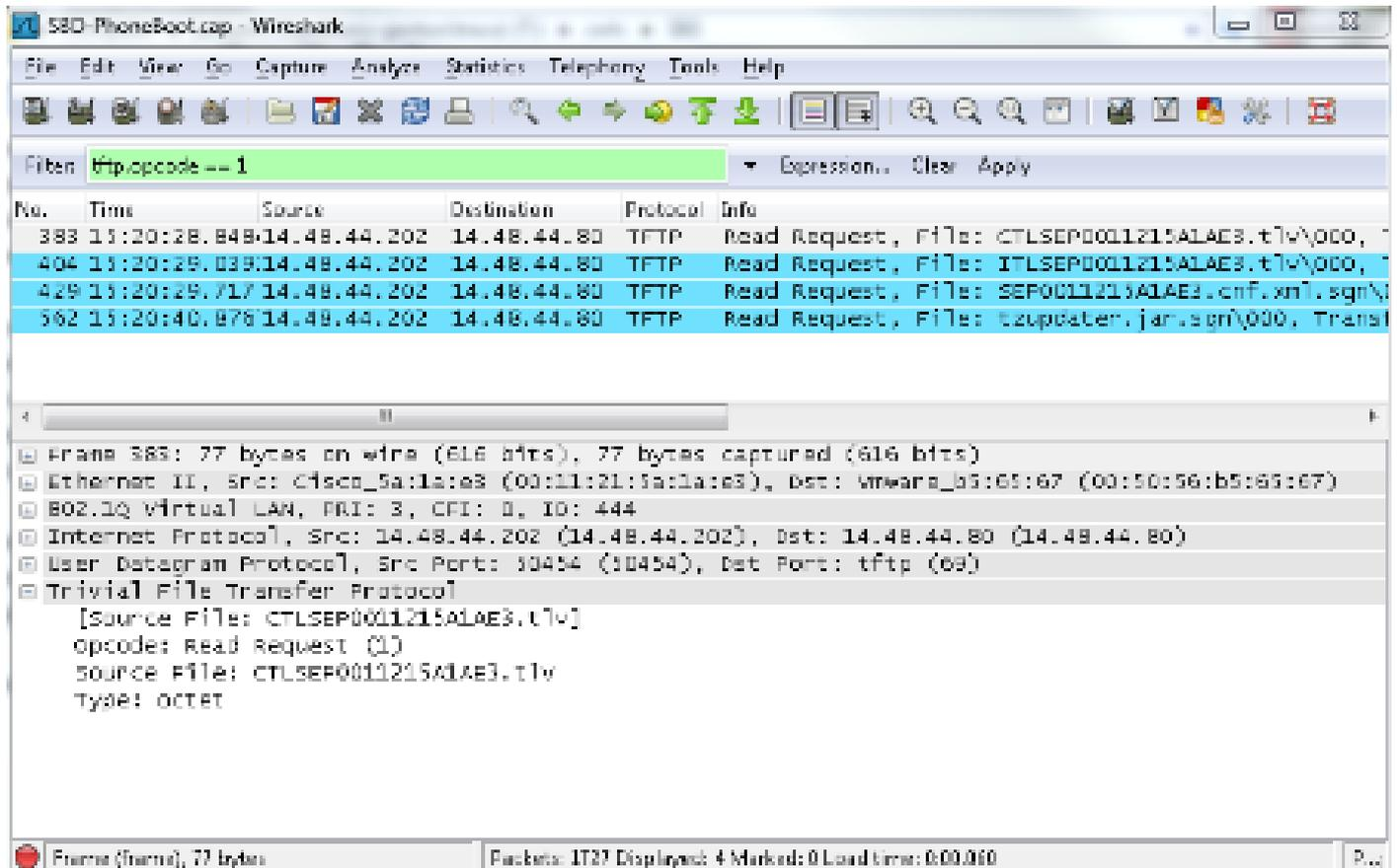
The image shows a Wireshark packet capture window titled "580-PhoneBoot.cap - Wireshark". The filter bar is set to "tftp.opcode == 1". The packet list pane shows four TFTP Read Request packets:
