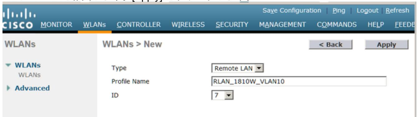
The screenshot shows the Cisco WLC configuration interface for creating a new Remote LAN. The page title is "WLANs > New". The "Type" is set to "Remote LAN", the "Profile Name" is "RLAN\_1810W\_VLAN10", and the "ID" is "7". There are "Back" and "Apply" buttons at the top right.
