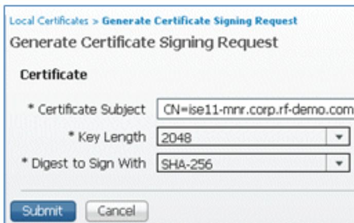
The image shows the 'Generate Certificate Signing Request' form in the ISE Administration console. The form has a title 'Generate Certificate Signing Request' and a sub-header 'Certificate'. There are three required fields: '\* Certificate Subject' with the value 'CN=ise11-mnr.corp.rf-demo.com', '\* Key Length' with a dropdown menu set to '2048', and '\* Digest to Sign With' with a dropdown menu set to 'SHA-256'. At the bottom of the form, there are two buttons: 'Submit' and 'Cancel'.
