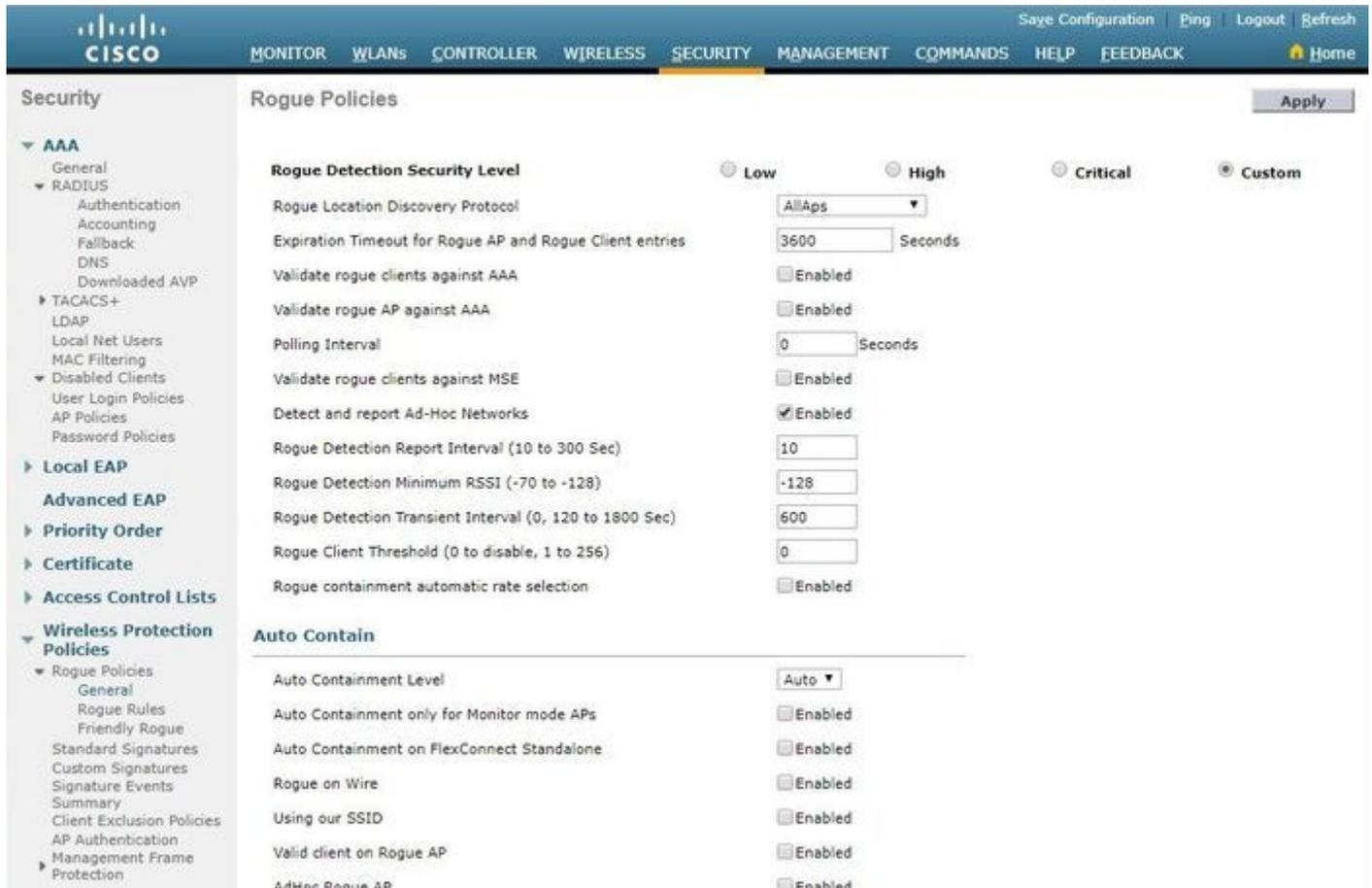
The screenshot shows the Cisco Security configuration interface for Rogue Policies. The 'Rogue Detection Security Level' is set to 'Custom'. The 'Expiration Timeout for Rogue AP and Rogue Client entries' is set to 3600 seconds. The 'Detect and report Ad-Hoc Networks' option is checked and enabled. The 'Auto Contain' section shows 'Auto Containment Level' set to 'Auto' and several other options are disabled.
