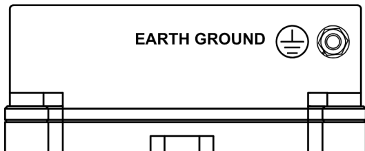
Figure 1 Earth Ground Connector on the Head of the Power Injector
