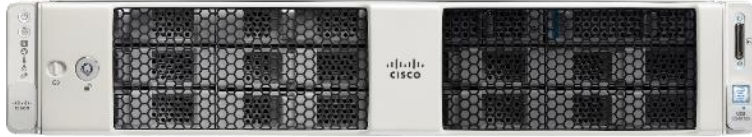
Figure 2. Cisco UCS C240 Rack Server
