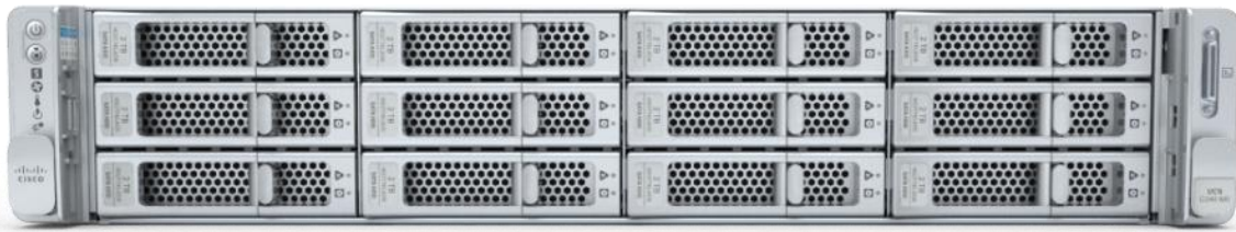
Figure 2. Front View: Cisco UCS C240 M6 Large Form Factor (LFF) server
