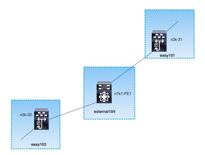
This topology shows only the border devices in the Data Center VXLAN EVPN and the core or edge router in the External Connectivity Network fabric.
