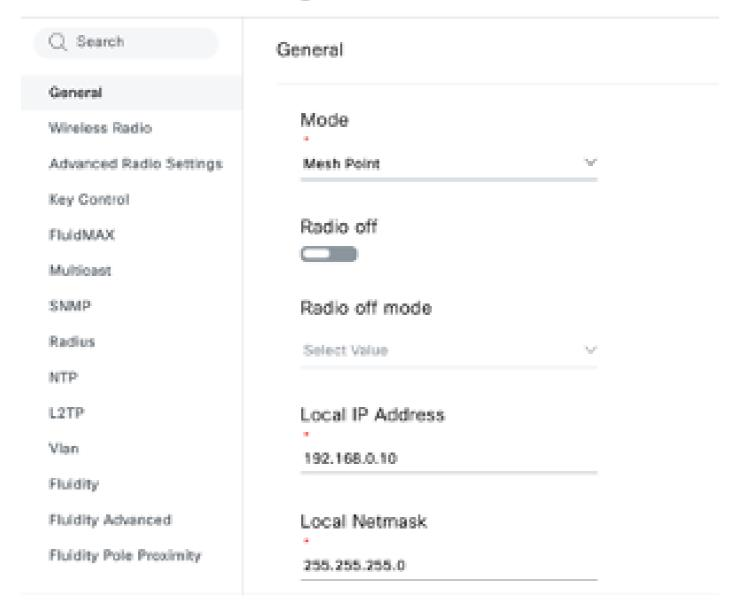
2. For a PTMP config, in the 'General Mode' section, the AP directly connected to the physical network (Radio A) is configured as a Mesh End and the two APs connected to the end devices (Radio B and Radio C) are configured as Mesh Points.
