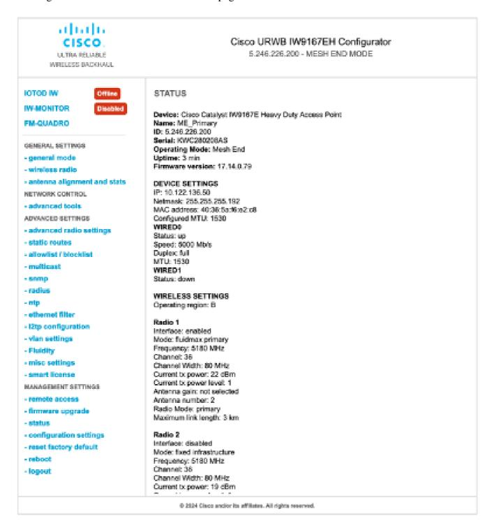
7. FM-Quadro page on the Mesh End radio can be accessed to check the layout of the PTP setup.
