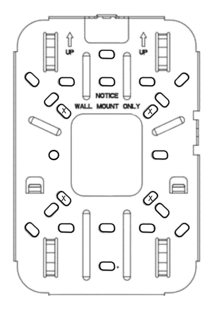
Step 2. Drill four pilot holes at the mounting locations you have marked.
