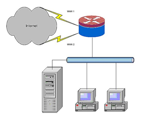
This document describes additional configuration to apply the Cisco IOS Zone–Based Policy Firewall (ZFW) to add stateful inspection capability to augment the basic network protection provided by NAT.
