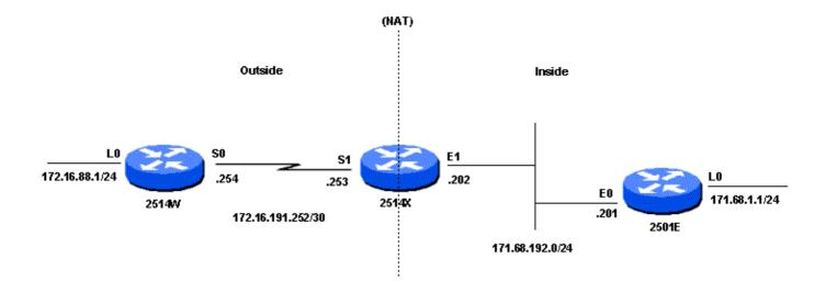
When ping is sourced from the Router 2514W Loopback0 interface (172.16.88.1) to the Router 2501E Loopback0 interface (171.68.1.1), this occurs:
