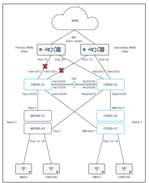
For the purpose of this test, ports TwentyFiveGigE1/0/1 and TwentyFiveGigE1/0/2 will be disconnected.
