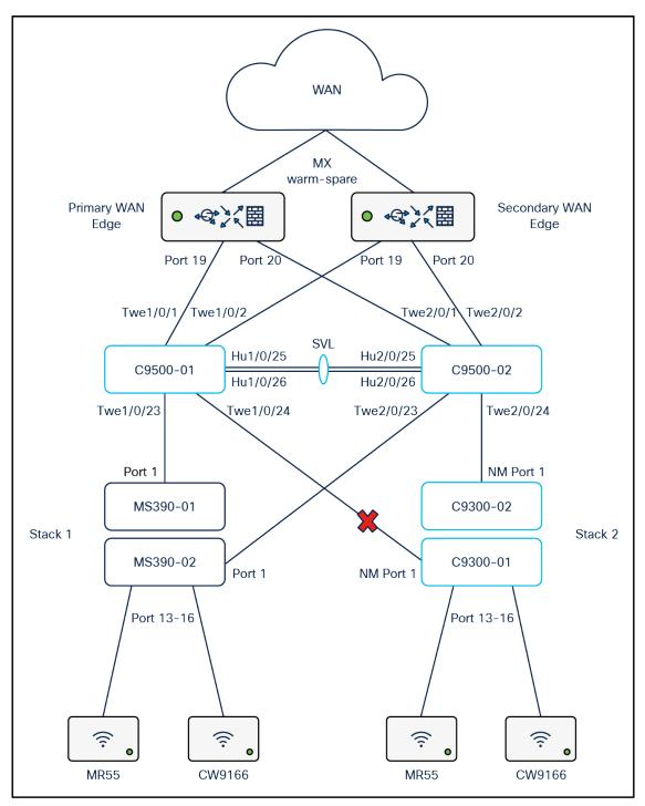
For the purpose of this test, NM Port 1 on C9300-01 (Master switch) will be disconnected.
