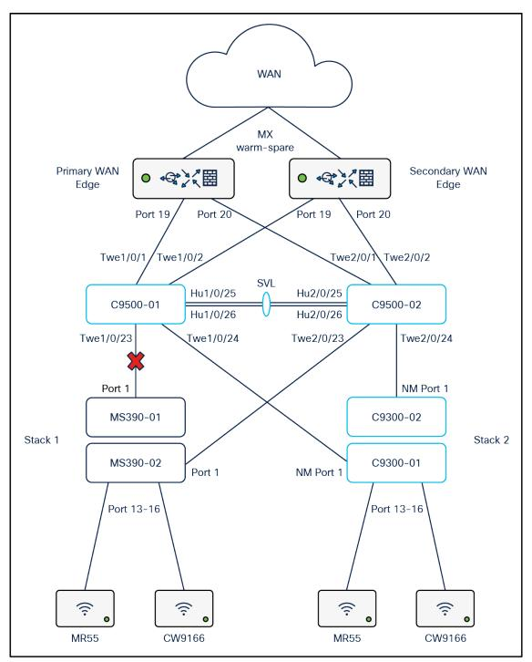
For the purpose of this test, port 1 on MS390-01 (Master switch) will be disconnected.
