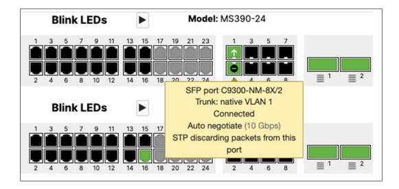
Note: Interface 26 is in STP BLK state (As expected since the Ether-channel is in FWD state)
