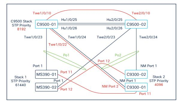
For the purpose of this test and in addition to the previous loop connections, the Bridge priority on C9300 Stack will be reduced to 4096 (likely root) and increasing the Bridge priority on C9500 to 8192.
