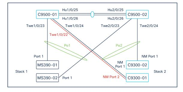
A loop was introduced by adding a link between C9300-01 /NM Port 2 and C9500 Core Stack / Port TwentyFiveGigE1/0/22 (Please note that for the purposes of this test, the interface has been unshut and configured as a Trunk port with Native VLAN 1 with STP guards on that interface)
