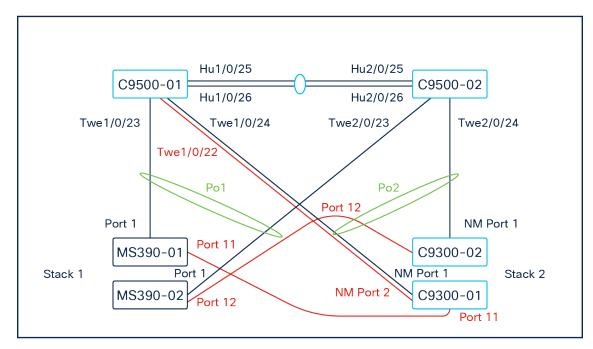
For the purposes of this test and in addition to the previous loop connections, the following ports were connected: MS390-02 / Port 12 < - > C9300-02 / Port 12.
