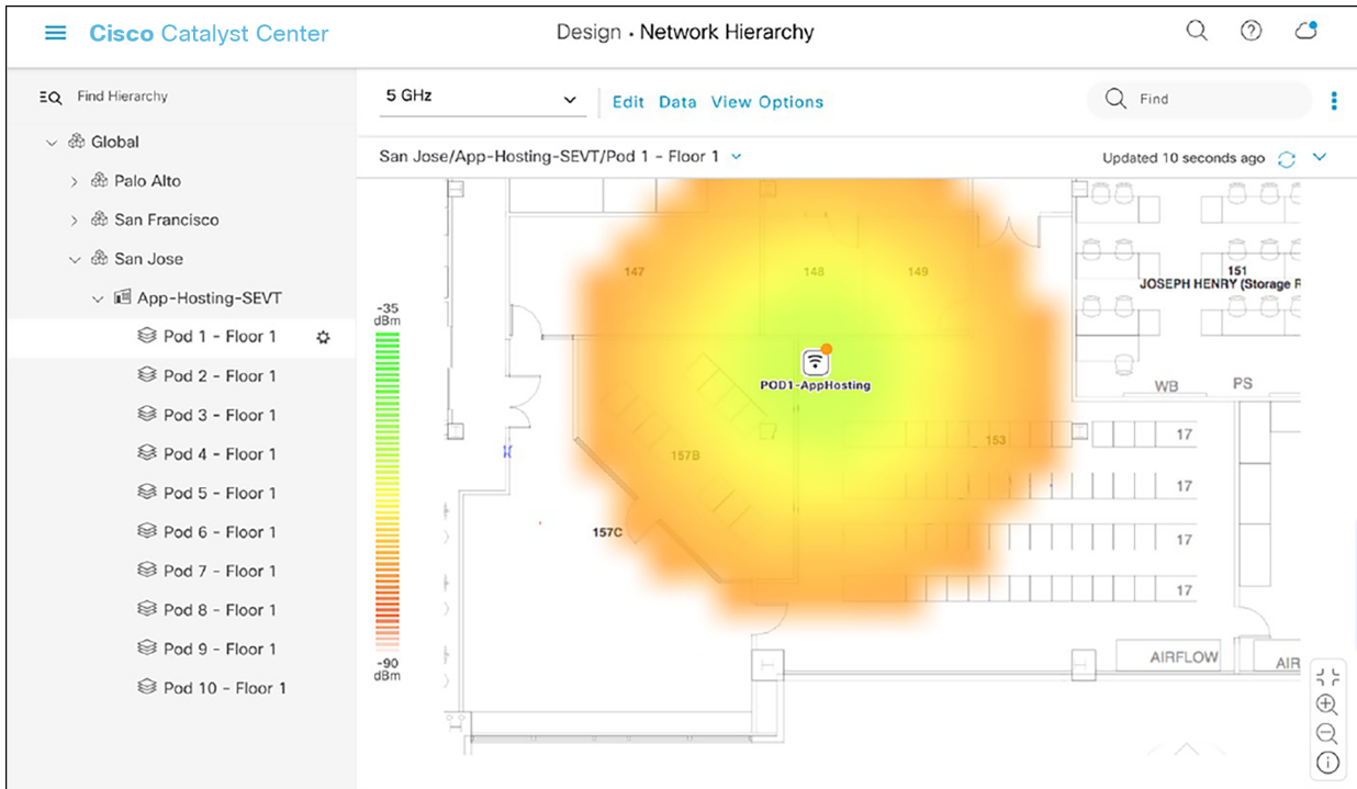
Figure 31. Network Hierarchy page, with heat map displayed after access points are positioned
