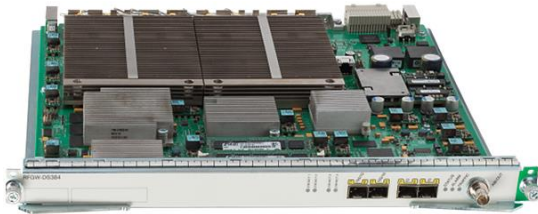
Figure 1. Cisco RF Gateway Downstream 384 Universal Edge QAM Line Card
