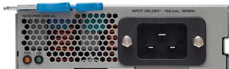
Figure 11. 3kW AC power supply
