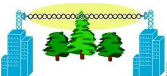
Figure 10 Typical Obstructions in a Fresnel Zone
