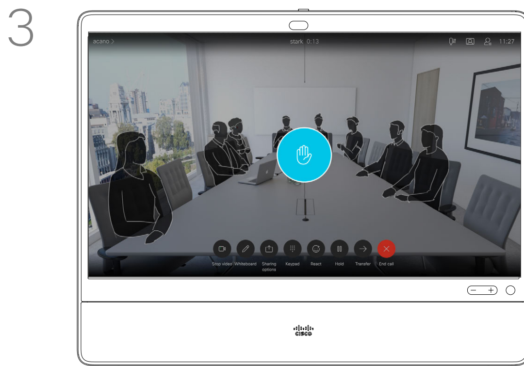
Hold your reaction until the timer is complete. If you stop your gesture before the timer is complete, no action is triggered.
