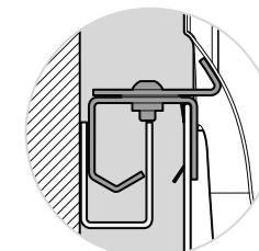
**Hold the screen close to the wall while lowering it onto the wall bracket. Check that the clips slide fully onto the top bracket.**
