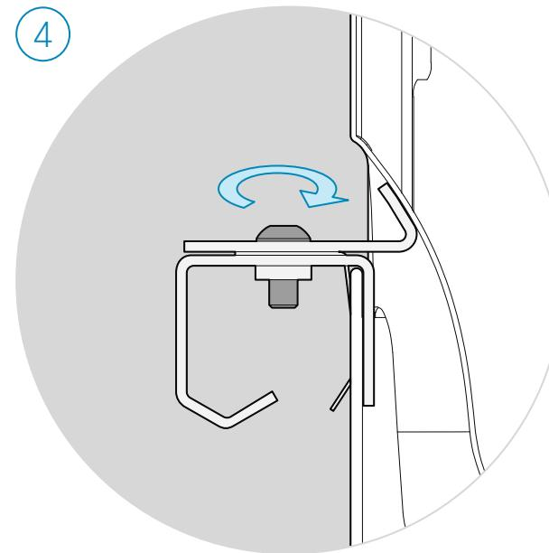
Tighten all screws and check that the clamp is securely fastened.
