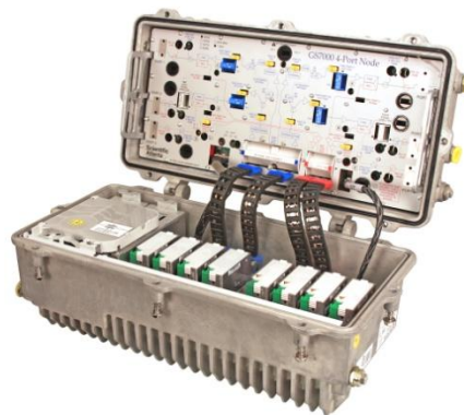
Figure 1. GS7000 4-Way Segmentable Node with 40/52 MHz Split
