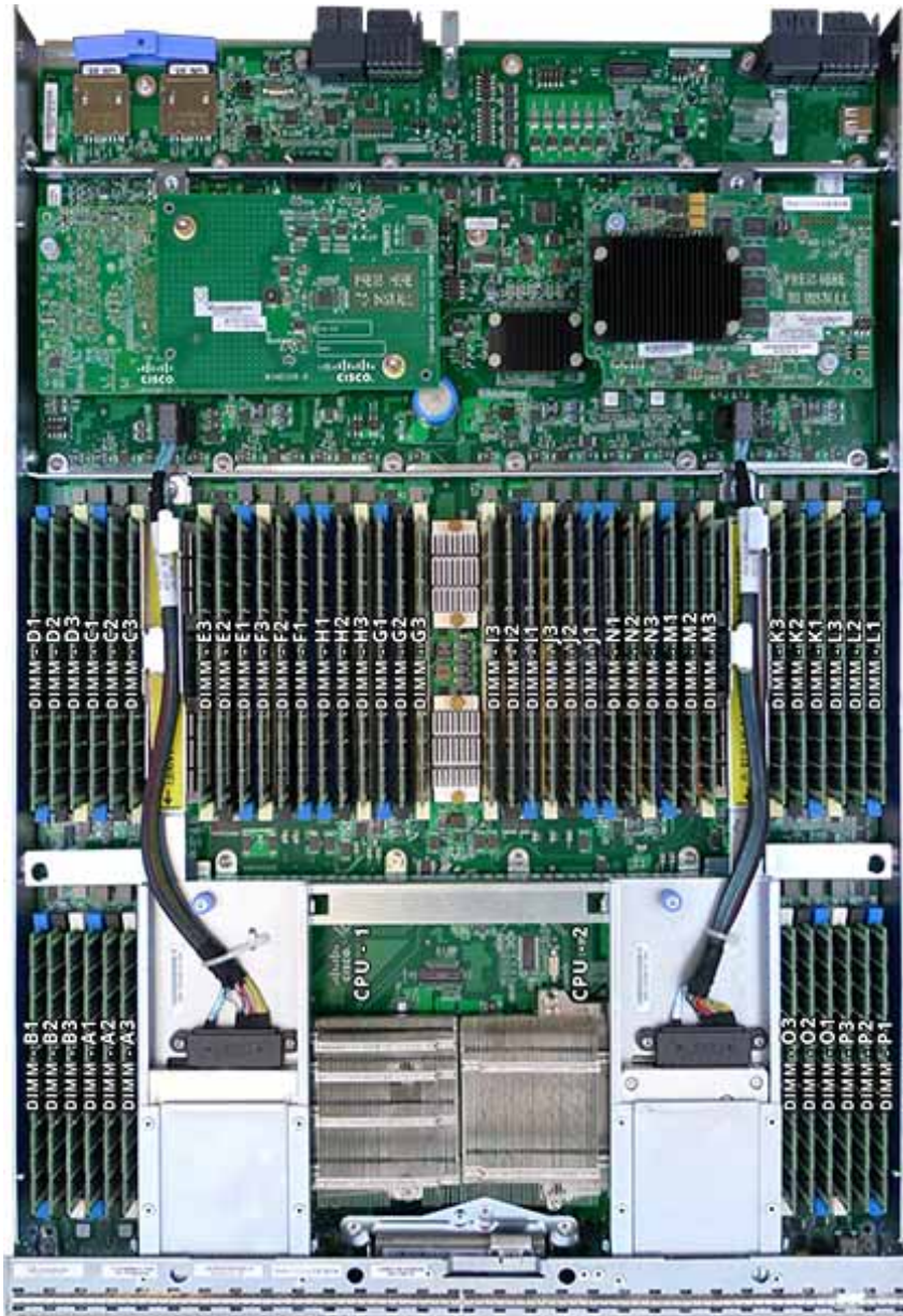
Figure 5 Top view of one of the two Blade Modules for B460 M4 E7 v4 (cover off)
